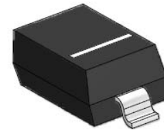
SOD-123 Gull Wing Lead
