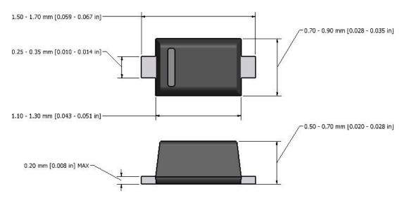
Note: Dimensions are exclusive of Burrs, Mold Flash & Tie Bar extrusions.
